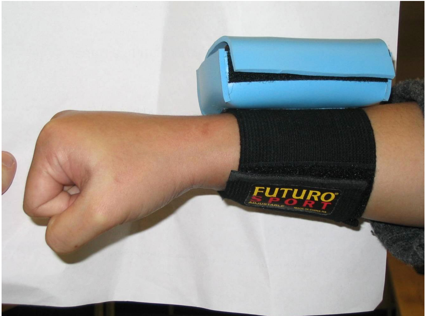
Fig. 9.20. A wireless motion monitoring device worn on the wrist of a user.
